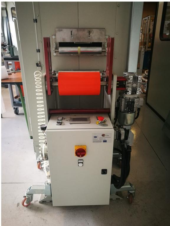
A pay off for tapes is provided to unwind the product to feed the stretching machine, the vaporizing oven, the cutting machine etc. The unwinding process will be tangential, controlled by AC motor. The motor may be operated in speed control or torque control for controlling the unwinding tension of the product.
